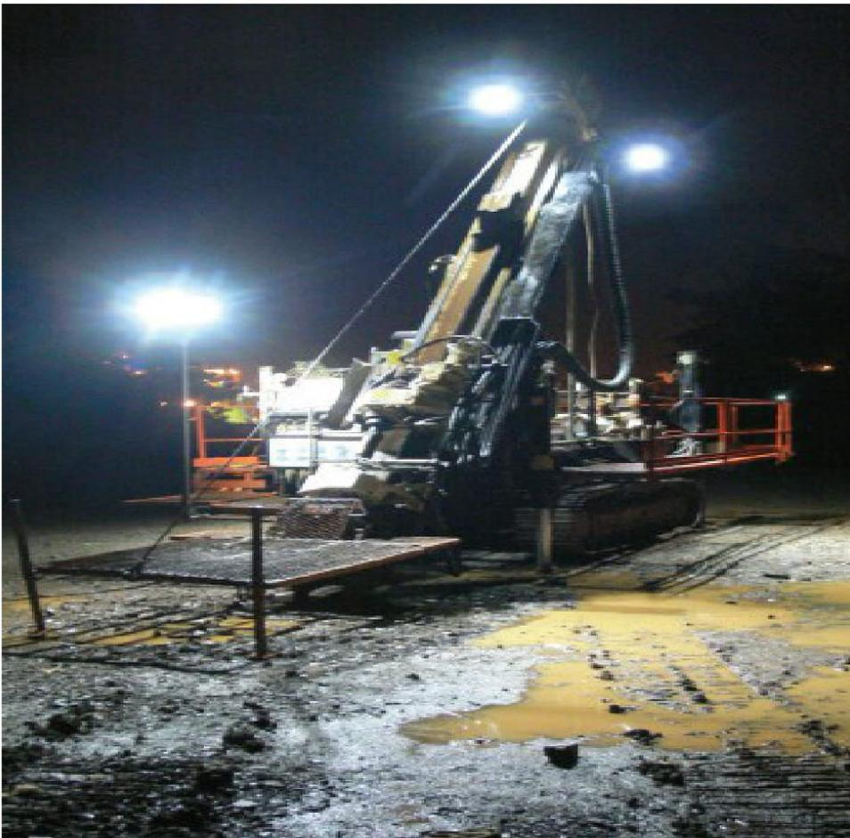
“The diesel generated 1 lighting plant ( 2 lights) are set up in one place to the front or side of the rig, this casts are large shadow to the opposite side of the machine creating a dark are which can cause trip hazards and lowered vision. The mounted lights removes almost all shadows around the perimeter (2-3 meters) all the way around the rig.”
